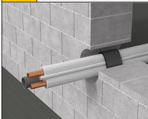
Fig.22 Bundle of combustible pipes / noncombustible pipes and cables in rigid wall with thickness A \geq 150 mm
