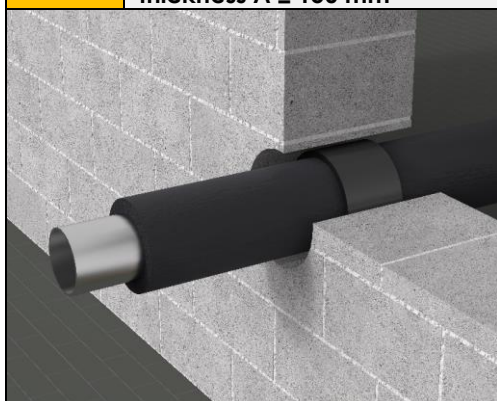
Fig.16 Non-combustible pipes with continuous insulation penetration seals with single row of band in rigid wall with thickness A \geq 150 mm
