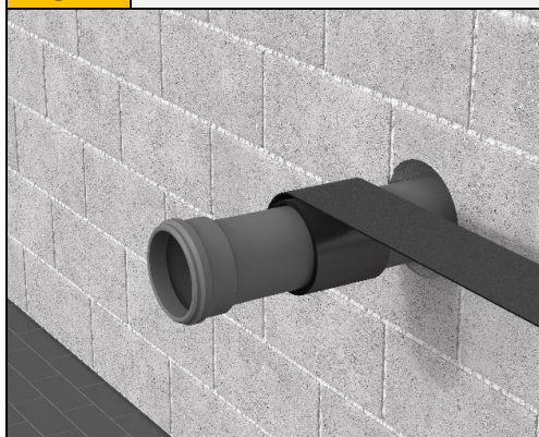
Fig.9 Combustible pipes penetration seals with single row of band in rigid wall with thickness A \geq 150 mm
