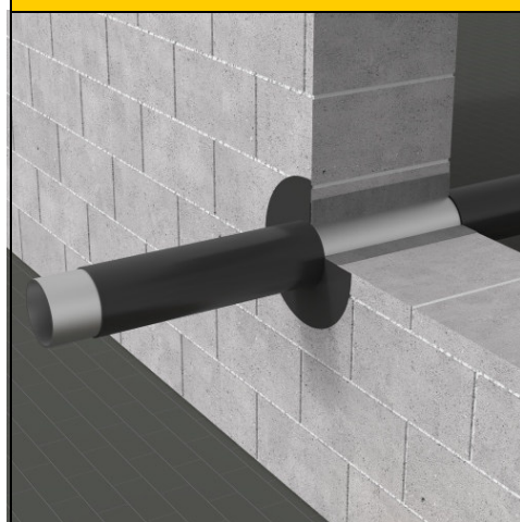
Fig. 1. Penetration with mortar filling in rigid wall
